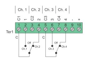
Wiring configurations shown here are examples. The wiring for your application may differ.
