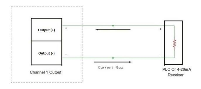
The above diagram shows the channel 1 output hooked to a 4-20mA receiver or PLC. The input resistance of the receiver can be up to 500 ohms. Anything higher and the current will be limited to below 20 mA since the maximum output voltage of the channel outputs is 10 volts.
