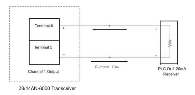
The above diagram shows the channel 1 output hooked to a 4-20mA receiver or PLC. The input resistance of the receiver can be up to 500 ohms. Anything higher and the current will be limited to below 20 mA since the maximum output voltage of the channel outputs is 10 volts.
