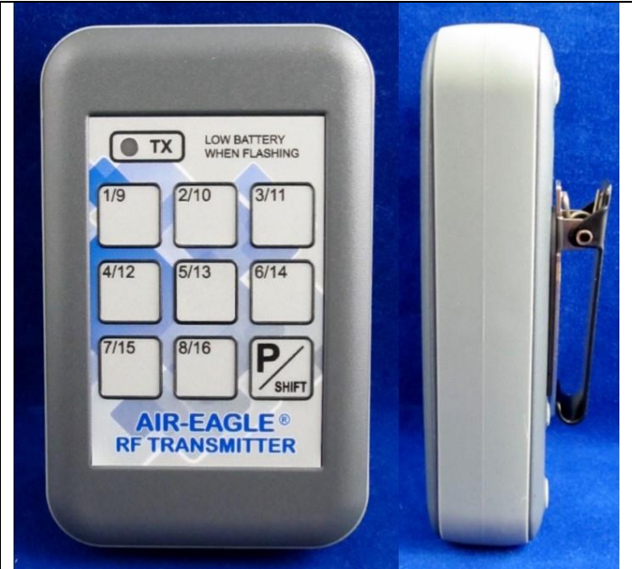
Dimensions: 4.71" L x 2.99" W x 1.12" D (Note – belt clip adds .43" to depth)
